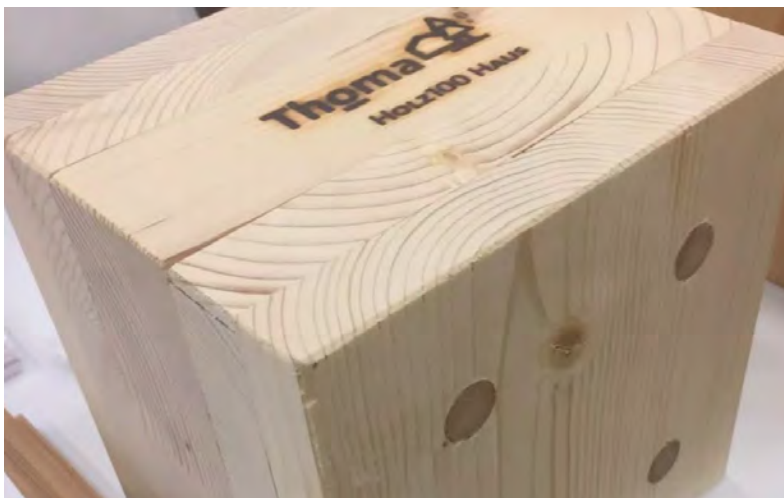
Figure 10 : Spruce cross-laminated timber, fastened with dowels made from beech wood, © Thoma, Austria
